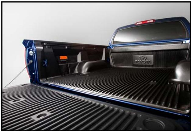
**Bed Liner**—Keeping Tundra’s bed looking new; the custom-fitted Bed Liner for Tundra not only protects against dents and scratches but also reduces mold and mildew by allowing drainage and increased airflow. The Liner, featuring a no-drill attachment system and made from high-density polyethylene copolymer, keeps loads from moving around in the bed. The Bed Liner also includes protection for the tailgate.
