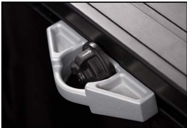
**Bed Cleat**—Add functionality with additional Bed Cleats. Designed specifically for the Tundra Bed Rails, they are constructed of sturdy die-cast aluminum, and each fully adjustable Bed Cleat is rated for a maximum load of 220 lb. Sold individually.
