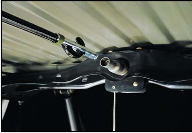
**Spare Tire Lock**—Secure your spare tire with a precision machined lock constructed of hardened steel with a zinc-nickel plating. It quickly attaches to the spare's crank-down tool receiver mechanism, and the key attaches to the crank-down tool in your Tundra tool kit.
