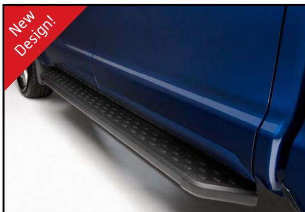
**Running Boards**—Not only do the Running Boards assist with entering your Tundra, they also help protect the lower body from road debris. Constructed from highly durable aluminum for corrosion-resistance, they feature a wide-step surface with rubber grommets to help ensure a secure footing. Engineered to mount securely to the Tundra's sides using existing mounting points.
